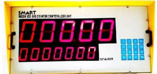
The instrument is single Microcontroller based, SWITCH MODE POWER SUPPLY UNIT ( SMPS ), KEYPAD for programming & counter setting & resetting, seven segment display unit for displaying running COUNT, TOTALISER, SET/PRESET COUNT. Use of HIGHLY DURABLE SENSING HEAD instead of conventional optical sensors & proximity switches gives better results, longer life in dusty (CEMENT INDUSTRY) and rough industrial atmosphere.
